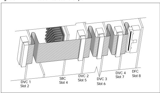
Figure 8 NAM II PEB Cable installation example
